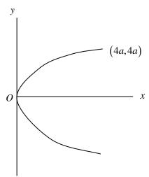
The equation of curve (as shown in the figure 4.16) can be written in parametric form as  $x = at^2 \Rightarrow dx = 2atdt$ ,  $y = 2at \Rightarrow dy = 2adt$ . Parameter, t varies from 0 to 2.
